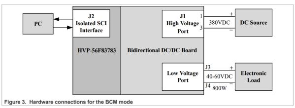
• Powering the boards: Power the platform by powering up the DC source.
