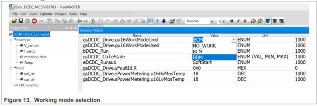
3. Click the drop-down menu of the bDCDC\_Run command and start/stop the converter.
