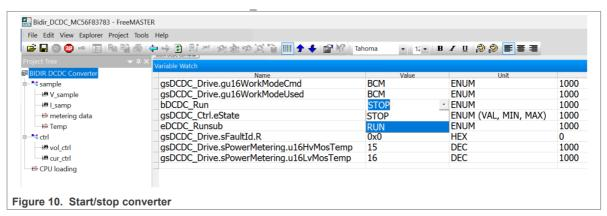
10. The low voltage port voltage ranges from 40 V to 60 V. You could change the low voltage port voltage by changing the macro: VLV\_BCM\_REF (Bidir\_DCDC\_MC56F83783 > source > bidir\_dcdc\_ctrl.h). The default low voltage port voltage is 56 V.
