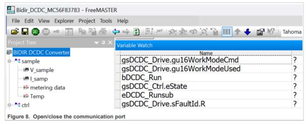
8. After the FreeMASTER communication is established, click the drop-down menu of the gsDCDC\_Drive.gu16WorkModeCmd command and select BCM.
