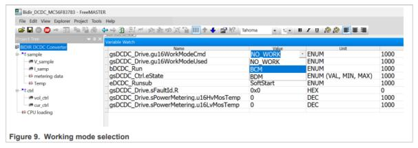
Click the drop-down menu of the bDCDC\_Run command and start/stop the converter.
