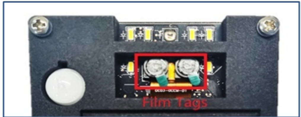
Figure 2. Protective film covering the two cameras: RGB and IR
