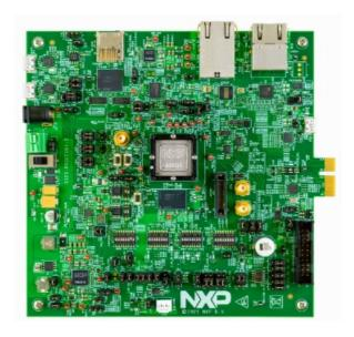
S32G is a vehicle network processor delivering high levels of real-time and applications processing, supporting CAN/LIN/FlexRay networking and Gigabit Ethernet interfaces with hardware acceleration and delivering a high level of embedded security and ASIL D functional safety capabilities.
