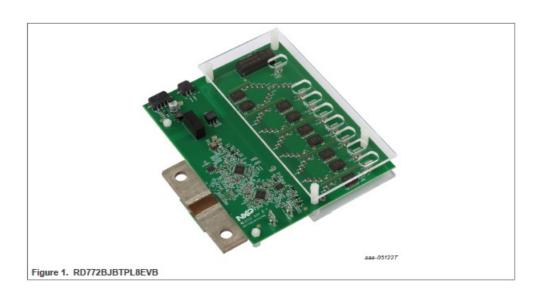
The RD772BJBTPL8EVB is a BJB reference design around two NXP MC33772C. The board is ideal to quickly prototyping the hardware and the software of a high-voltage BMS. This document describes the RD772BJBTPL8EVB features.
