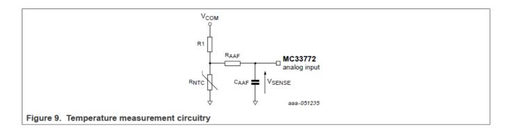
• Figure 9 describes the temperature measurement circuitry.
