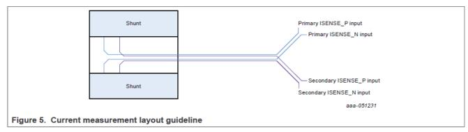
• In a real application, the current measurement paths must be independent. The connection points to the sense element of the shunt resistor have to be redundant as shown in Figure 5.
