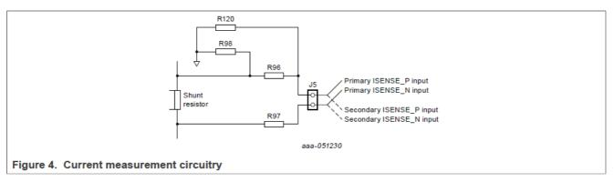
• Then, a voltage source can replace a high-current source to validate the current measurement feature. Figure 4 describes the current measurement circuitry.
