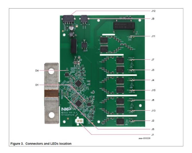
• The Figure 3 lists the connectors and the LEDs available on the RD772BJBTPL8EVB.
