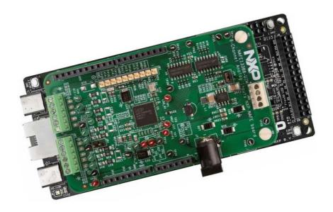
Software-configurable analog input solution with versatile sensor support, real-time diagnostics and reliable wired connectivity enabling high-precision sensing and edge
