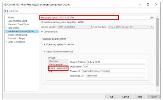
From this panel, the user can update the model Board Parameters like device address, user name, password, and download folder.
