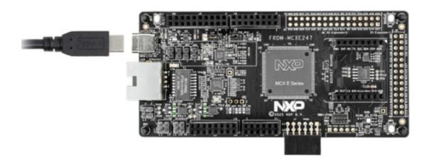
1. Connect the FRDM-MCXE247 board to a PC using the USB Type-C® cable
