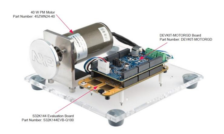
S32K144 development kit for 3-phase PMSM and BLDC motor control
