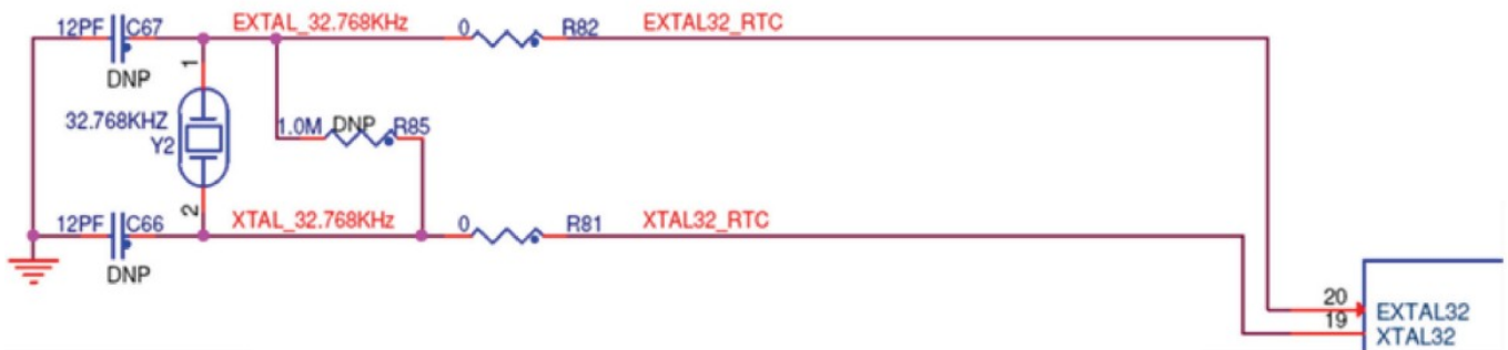
Figure 7. 32.768 kHz crystal for RTC
