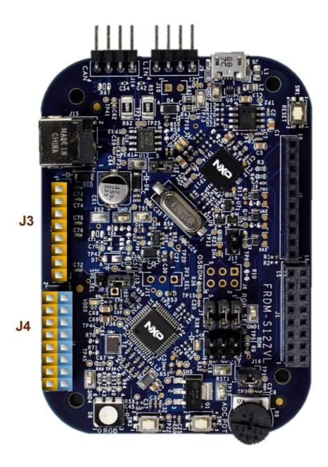
$\label{eq:compatibility} \textbf{Arduino Compatibility} \\ \textbf{The internal rows of the I/O headers on the DEVKIT-ZVL128 are arranged to fulfill Arduino} \\ \textbf{shields compatibility} \; .$
