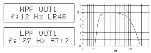
In the "CROSSOVER" menu, each setting in the "MAIN CONTROL" changes the parameter in editing, between output, filter type, frequency and attenuation / topology.
