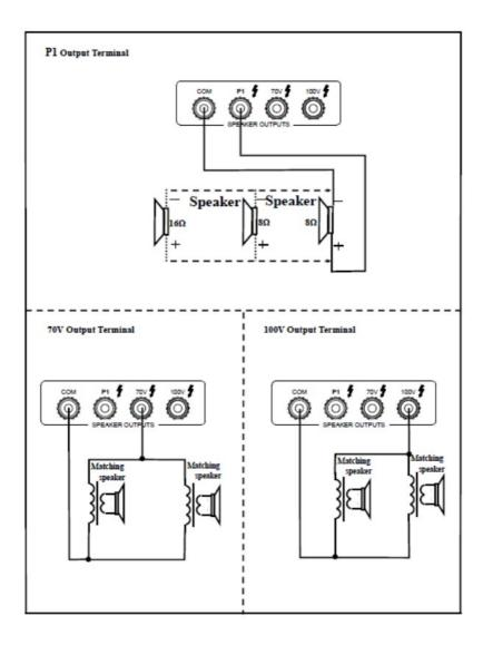
**Note:** The four outputs are connected using the following methods: COM-P1, COM70V, and COM-100V. Only one set of output terminals can be connected, and the speaker connected to COM-P1 cannot be linked to COM-70V and COM-100V; otherwise, the speaker may be burned.
