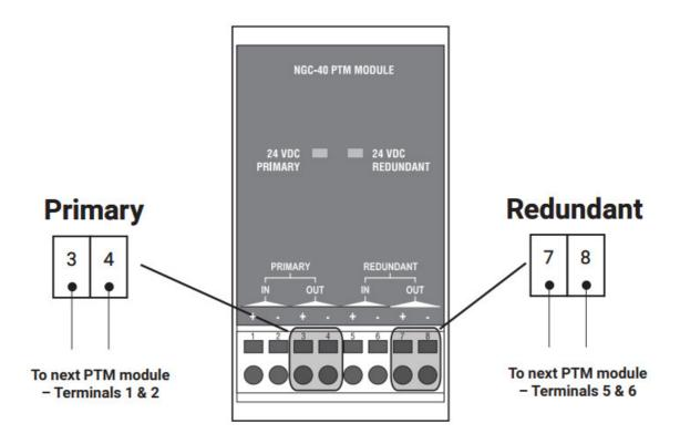
Note: The primary and redundant 24 Vdc outputs each support only one additional NGC-40 PTM module
