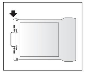
**REMOVAL:** Push the module upwards to disengage the clip, then rotate the module toward you.
