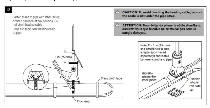
• Screw box onto stand until it stops. Do not overtighten.
