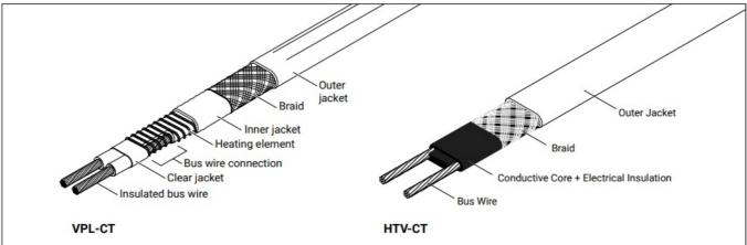
Allow approximately 24 in (60 cm) of heating cable for installation. For VPL, cut cable 12 in (30 cm) from bus indentation. • Cut off heating cable end at about 45° for easier insertion.
