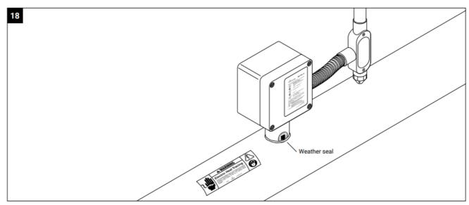
**WARNING:** Explosion Hazard- Substitution of Components May Impair Suitablity for Class I Division 2 (Zone 2)
