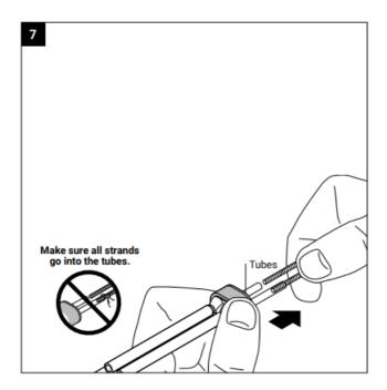
Push core sealer onto the heating cable to the mark made in step 6.
