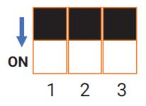
Push the button to ON (as the arrow indicates) side will connect the corresponding resistor in.
