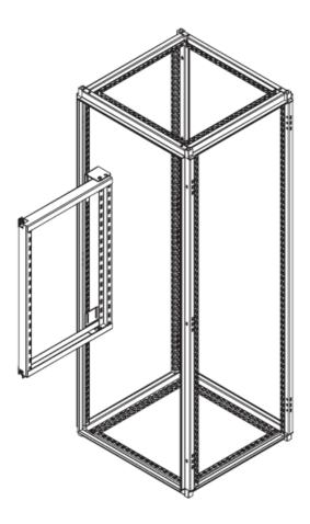
**NOTE**: The swing frame can be mounted using the M5x10 self–tapping screws (item 14), or it can be mounted using the M6x16 screws (item 16) with the M6 cage nuts (item 10).
