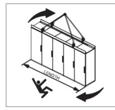
Twisting or tipping cabinet set can cause injury and damage. Minimize tipp ing by using recommended Lifting
