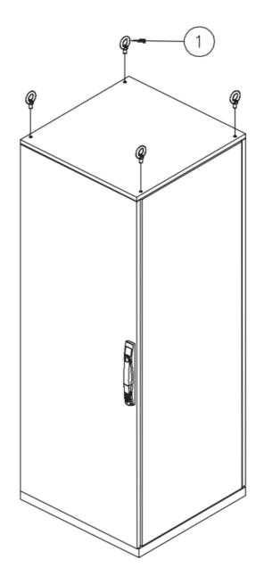
Lift Angle For Lifting Side-To-Side Mounted Cabinets
