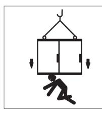
Loose fastener can cause cabinet(s) to fall and seriously injure. Torque fasteners to 30 in–lbs.
