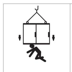
Loose fastener can cause cabinet(s) to fall and seriously injure. Torque fasteners to 30 in–lbs.
