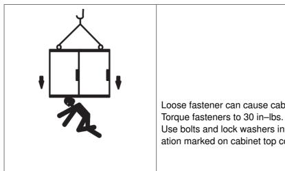
Loose fastener can cause cabinet(s) to fall and seriously injure.
