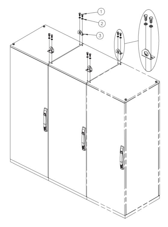
Lift Angle For Lifting Front–To–Back Mounted Cabinets (Catalog Number PJLBFB)
