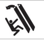
Falling Lift Bars can cause serious injury. When not in use, lay Lift Bars flat
