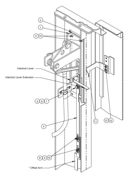
\* Parts of Lock Release Mechanism
