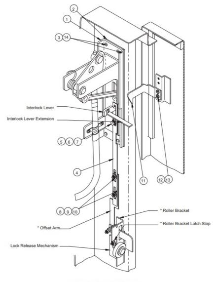
\* Parts of Lock Release Mechanism
