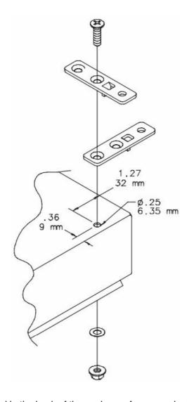
Mounting holes have been provided in the back of the enclosure for convenient mounting trough the enclosure. Attach enclosure to wall or other structure using customer supplied 3/8 inch or M8 fastener, flat washers, and nuts. To insure proper sealing and enclosure protection rating, use the provided sealing washers. Install sealing washers inside the enclosure with rubber face against the enclosure.
