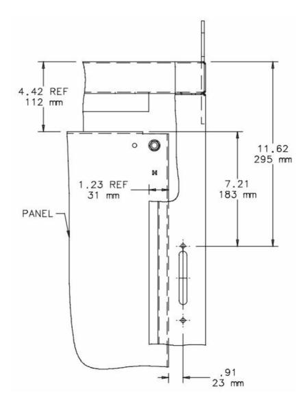
**NOTICE:** To maintain the environmental rating of this enclosure, install in any opening, only listed or recognized disconnect devices, external mounting feet, or conduit hubs that have the same environmental rating as the enclosure. Install in compliance with the installation instructions of the device.
