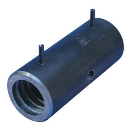
The side fill horizontal T-Series sleeve has vent holes located 90 degrees from the tap hole to facilitate side fill installations when the interferences of the structure will not allow top filling. The vent holes are added to horizontal sleeves to reduce air entrapment and help ensure proper filling of the sleeve.
