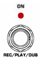
Engages the delay effect. When using LOOP mode, it controls REC/PLAY/DUB.
