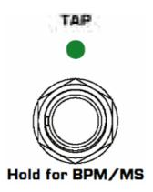
Tap this foot switch to adjust the speed and delay sub-division. You can set the target subdivision by TIME 1 and TIME 2 knobs, then TAP this foot switch to adjust the speed, the DELAY 1 and DELAY 2 will change the delay time according to the current sub-division note signature. Hold this foot switch for 2 seconds, to switch current delay time between MS or BPM.
