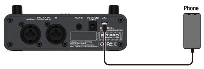
When connecting your smartphone to B-7 PRO for the first time, it may show two options on the phone's screen for you to choose. Please select the "USB headphones device". Or, you can check and setup "Connected To Headphones" as below.
