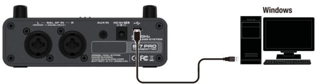
After you install the NUX ASIO Driver to you computer, you can connect the TX of B-7 PRO to your computer with a USB cable, you will find it as a USB audio device as below. Then you can start to record.
