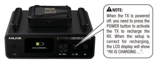
2. Recharge the RX with a 5V/O.5A adapter via the USB-C port.
