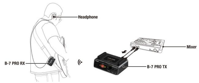
4. You can rotate the knob on TX's panel to adjust the output volume, and press the knob to adjust the Pan of output UR.
