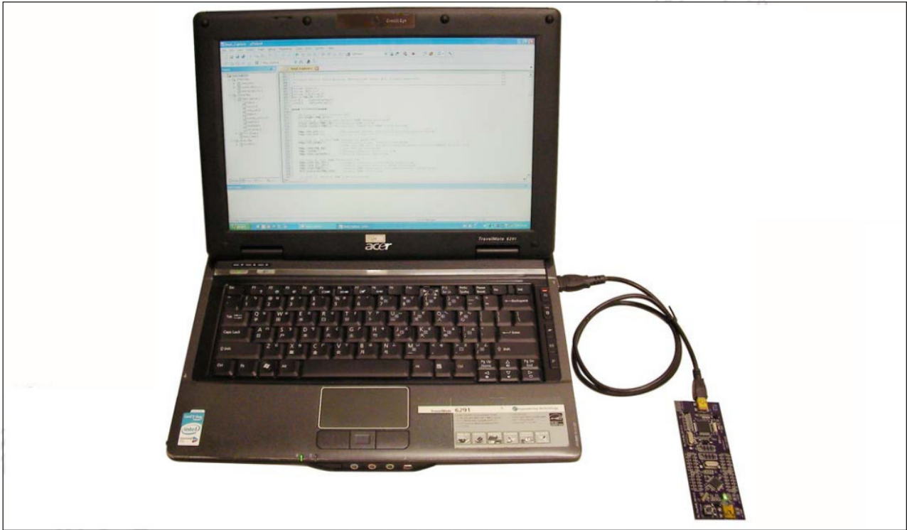
Figure 4-1 NuTiny-SDK-NUC122 Hardware Setup
