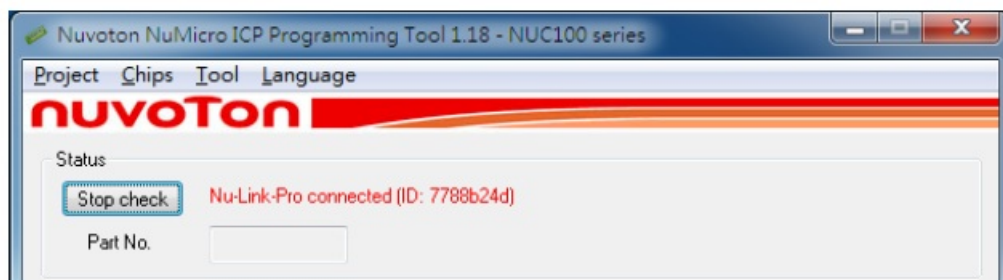
Figure 4-8 Nu-Link Adapter Connected with No Target Chip Detected
