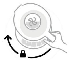
5. Place the pitcher onto the motor base — handle facing to the right of the blending control panel, never towards the back — and gently twist clockwise so it locks in place. When you hear the click, it's locked and ready to blend.
