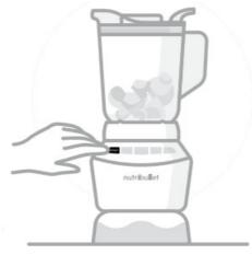
7. To start blending, select a speed or the EXTRACT program on the blending control panel. This program will turn off automatically. Buttons will illuminate while in use. **NOTE:** Proceed to the blending control panel chart on page 20 for speed definitions.
