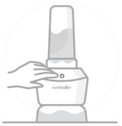
8. When you have reached your desired consistency, pause/stop the appliance by pressing **POWER** or the speed you selected and wait for the blades to stop turning. The unit will enter idle mode. The **POWER** button will remain illuminated.
