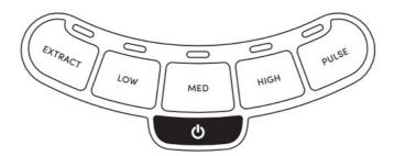
The power button actuates the master power of the appliance. When pressed, this button lights up to indicate the motor is powered on, and the other functions can be used. Always turn the master power off and unplug the unit when the machine is not in use.
