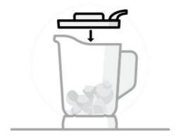
4. Place the pitcher lid with a vented lid cap attached to the pitcher, making sure it's aligned to the handle.
