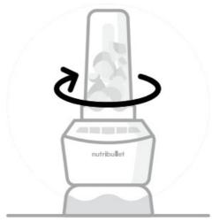
6. Turn the cup upside down and place it onto the motor base, gently turning the cup clockwise to lock into the motor base.
