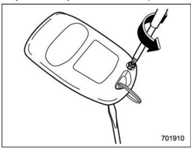
1. Remove the small phillips screw located on the back side lower left corner of the transmitter.
