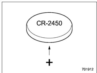
Remove the circuit board from the bottom half of the case and remove the battery and replace with new one. Be sure to observe the (+) sign on the old battery before removing it to ensure that the new battery is inserted properly (battery "+" should be pointed away from the transmitter circuit board on battery).
