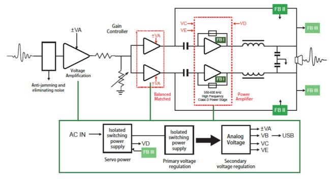
Modern floating voltage technology causes the voltage to change in accordance with the strength of the incoming music signal.
