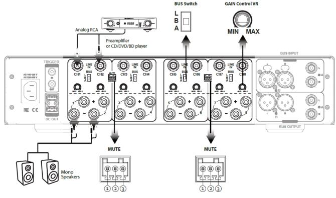
1 and 2 short CH1 and CH2 channels muted. 3 and 2 short CH3 and CH4 channels muted.
