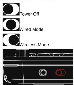
\* In the wired mode, it is necessary to use a data cable to connect with the device.
