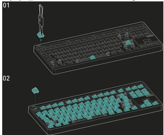
\*When installing a switch, please make sure to aim the switch pins correctly so both pins are aligned with a hole on the socket simultaneously before insertion, failure to do so could easily damage the pins.
