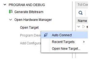
**Step 3:** If the device is detected successfully, to program the device, right-click on the target device "xc7a35t\_0" and select "Program Device" as shown below.
