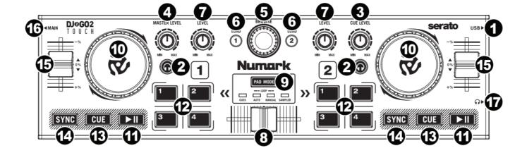
1. Mini-USB Port Plug the included mini-USB cable into this port and into the USB port of your computer to power DJ2GO2 Touch. DJ2GO2 Touch is class-compliant, so it is "plug-and-play" – no separate driver installation is
