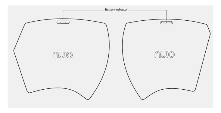
Alternatively, you may check the battery level by pressing the Battery Indicator button on the bottom of each keyboard. The button lights up to indicate the level of charge:
