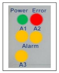
**Problem:** Analyser in fault condition. Analyser display and Analogue output will read a fault value. (28% O2 displayed and 22mA)
