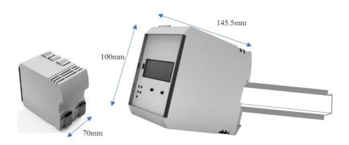
Mount the SIL O2 Analyser onto 35mm DIN rail as shown. Any Trunking/wireways above and below the Analyer when in situ, must be positioned so that there is a minimum of 30mm clearance between such trunking and the Analyser connection terminals.
