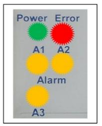
**Problem:** If the sensor is disconnected, this would ordinarily cause relays R1, R2 and R3 to deenergise. Analyser display and Analogue output will read a fault value. (28% O2 displayed and 22mA output) Solution: Check Sensor wiring and connect the sensor to the Analyser. After approximately 30 seconds, the Analyser will reset and the Red LED should extinguish.
