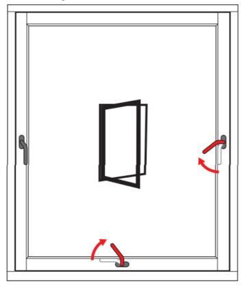
Turn the left and lower handle to open the window. Right hand hung
