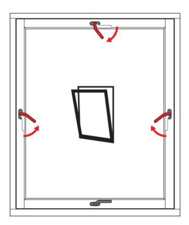
Turn the right, top and lower handle to open the window. Left hand hung
