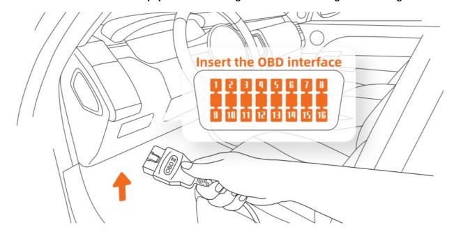
**OBD-11 Connector and Pinout**
