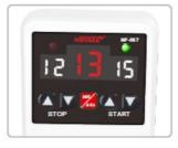
When "stop temperature" < "start temperature", the temperature controller is in the "high temperature start" state as shown in the figure. At this time, the green light is on, and the socket is powered. It is mainly used for cooling, such as turning on the air conditioner, exhaust fan, etc.
