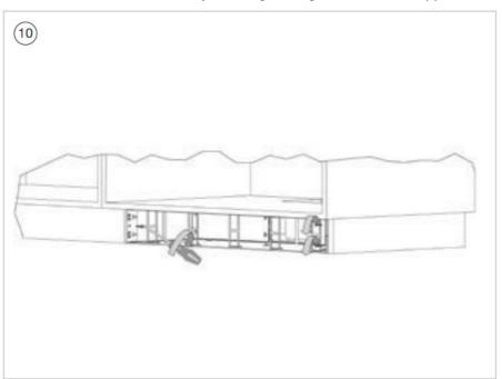
11. Make the connection between the cooker hood and the re circulation box with drainage ducts (not included).
