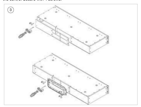
4. Connect the position of a connection opening at the rear corner: mount the plate at the centre read, with slots facing the corner. Secure with 4 screws.
