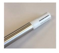
• Step 2: Remove the tip by turning it counterclockwise.
