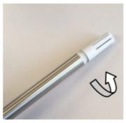
• Step 3: Without the tip, the sensor will be exposed. Remove it by puling it forward to disconnect it.
