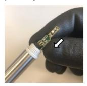
• Step 5: Place the protection tip again and turn it clockwise to secure it to the device
