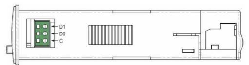
The table below helps you connect the RS485 communication interface connectors
