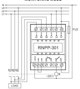
**FU1**, **FU2** – fuse 6.3 A (circuit breaker), **K** – contactor.
