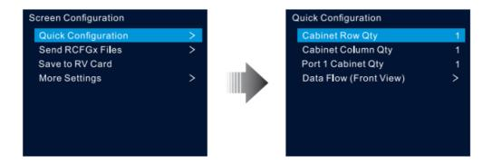
Step 5 Rotate the knob to select Port 1 Cabinet Qty to set the quantity of the cabinets loaded by Ethernet port 1.
