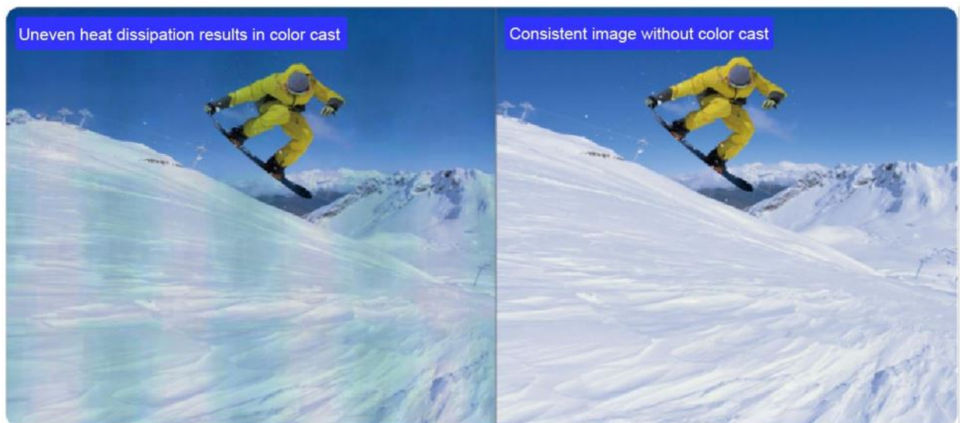
Figure 3-9 Before and after thermal compensation
