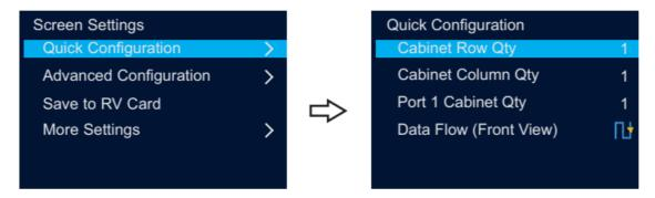
Step 4 Rotate the knob to select Port 1 Cabinet Qty to set the quantity of the cabinets loaded by Ethernet port
