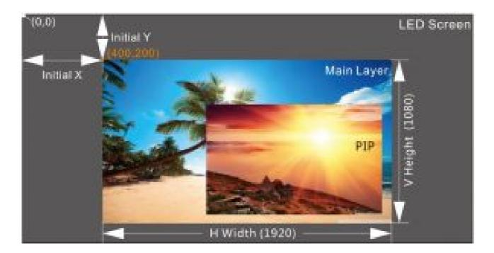
The greater the priority number is, the higher priority the layer has. In the above example, the main layer priority is 1 and the PIP priority is 2.
