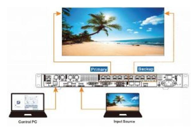
Log in to NovaLCT, and then go to Screen Configuration> Sending Card. Under the Sanding Card tab, set the backup between Ethernet ports in the Redundancy area.
