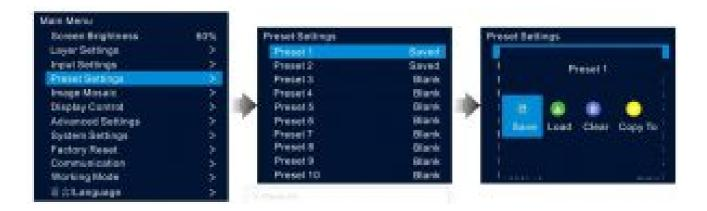
Save: Save the current layer settings to a specified preset. If the target preset is a saved one, it will be
