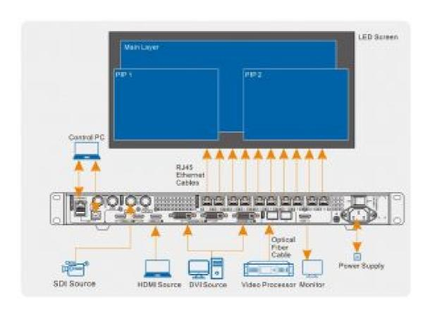
• Work as a fiber converter for long-distance transmission
