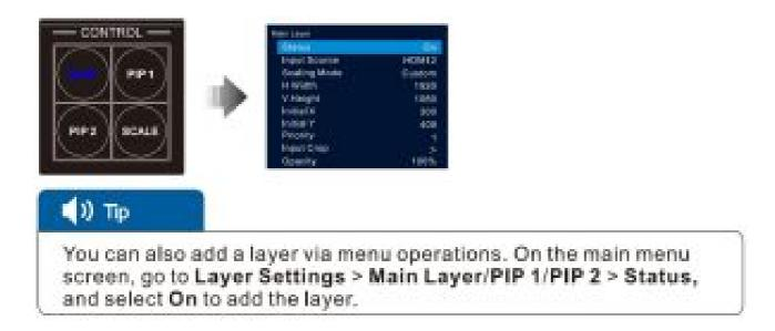
**Step 3** Rotate the knob to select Input Source and press the knob to open the input sources pane. Select the desired input source for the layer and press the knob to confirm.
