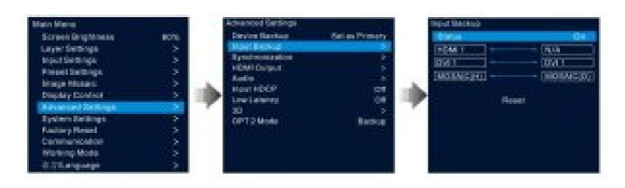
**Step 1** Rotate the knob to turn on the input source backup function. On the left are the default input sources, and on the right you can set the backup sources.
