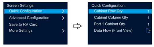
Step 4 Rotate the knob to select Port 1 Cabinet Qty to set the quantity of the cabinets loaded by Ethernet port 1.
