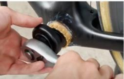
You can also screw it with the socket and the torque wrench
