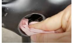
Grease the frame and the bottom bracket thread
