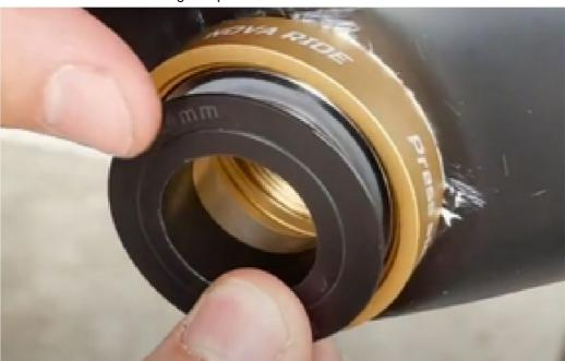
Screw the left cup (thread side), on the non drive side, clockwise first by hand and then using the Nova Ride key
