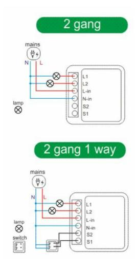
Note: The ZigBee Switch must be powered up by N and L wires
