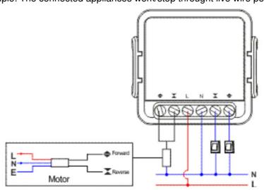
Note: The ZigBee Switch must be powered up by N and L wires
