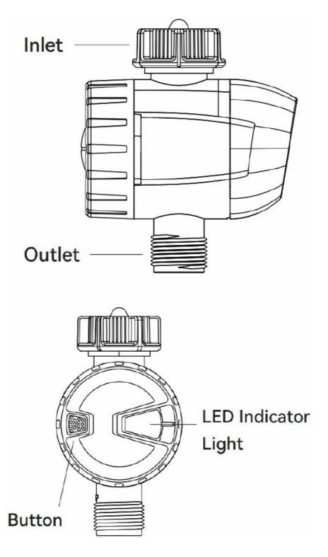
• Insert 3\*AAA batteries first, then press and hold the rubber button until the blue LED starts to flash quickly, which means the device is ready to connect.
